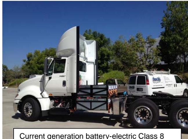
Current generation battery-electric Class 8 truck in recent tests, showing large number of batteries required. Source: TransPower
