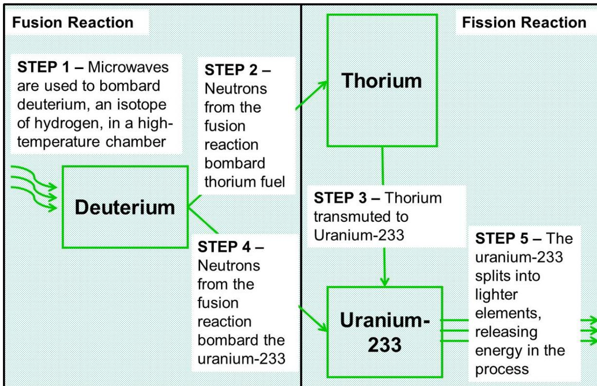
Figure 1. Illustration of Hybrid Thorium Reactor process.
