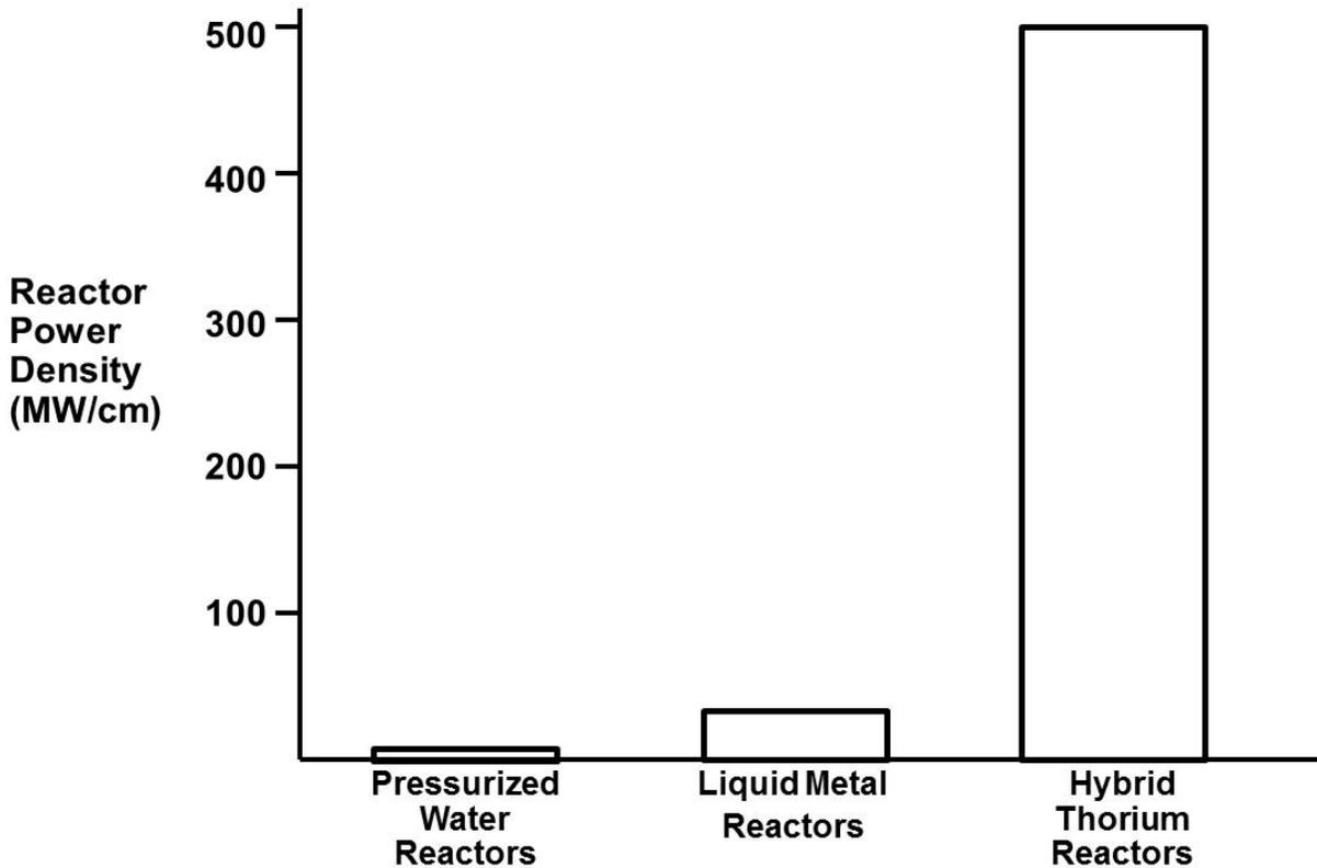
*Figure 3. Hybrid thorium power density as compared with conventional nuclear reactors.*
