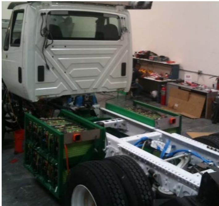
The photo to the right shows TransPower's first prototype electric Class 8 truck tractor during the latter stages of assembly in 2011.
